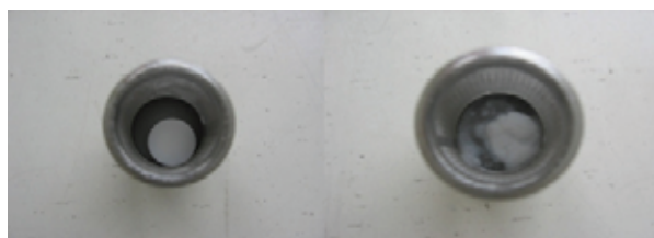
Figure 5. Tablets appearance after in vitro dissolution test (left- formulation F8; right- formulation F12).
