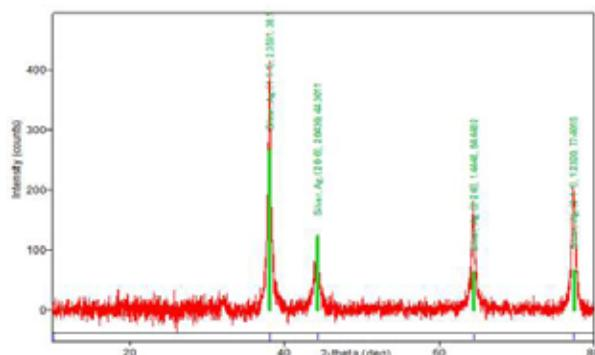
**Figure 2.** XRD pattern of the crystal structures of AgNPs synthesized from *Prunus dulcis L.* leaf extract
