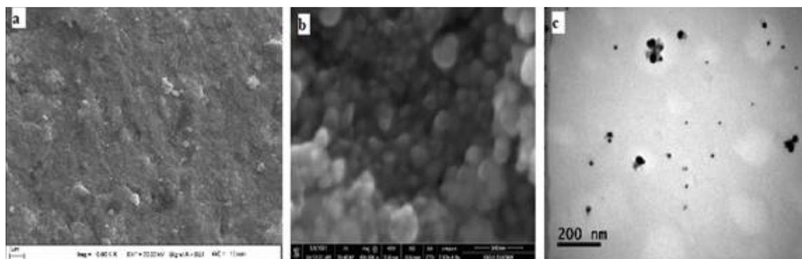
**Figure 4.** Micrographs of AgNPs synthesized from *Prunus dulcis L.* leaf extract a. SEM, b. FESEM, c. TEM images
