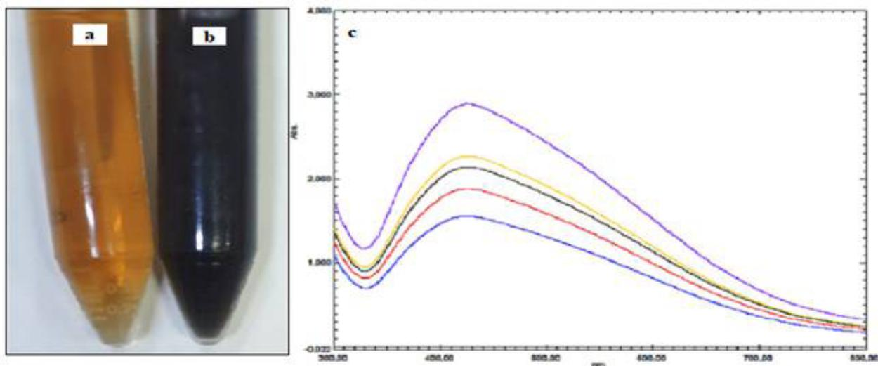
**Figure 1.** a. Leaf extract b. Dark brown color change due to the Formation of AgNPs, c. UV-vis. indicating the presence of AgNPs synthesized from *Prunus dulcis* L. leaf extract spectra.
