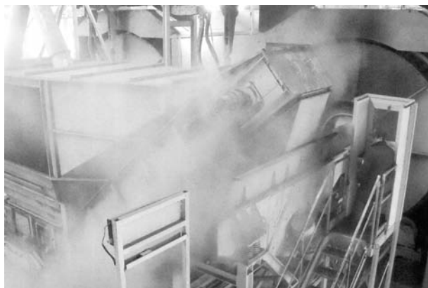
Figure 1 - Loading of a rotary kiln for lead fusion
