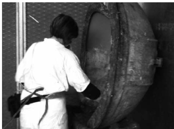
Figure 1 - Hand lay-up of styrene resin of a medium-sized piece at site A. The worker is wearing gloves and a dust mask. The small bag at the waist is a pump for air sampling (data not reported here).
