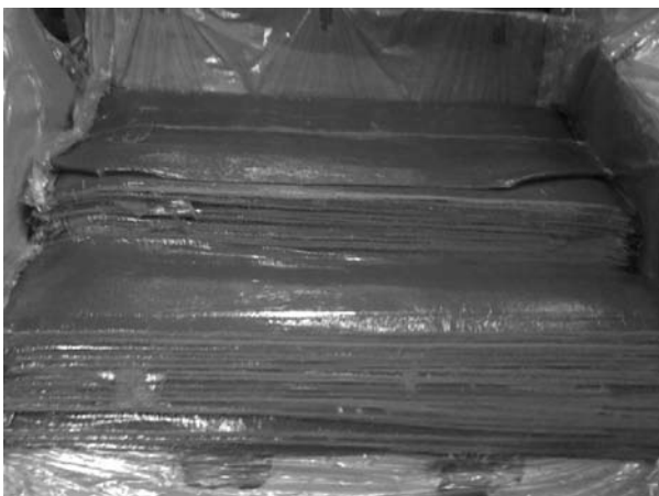
Figure 2 - Foils of moulding compound as delivered by the supplier at site B
