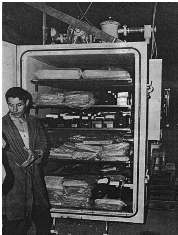
Figure 1 - Florence; FNCL: flooded library materials that were enclosed in plastic bags and treated with EtO inside the fumigator
