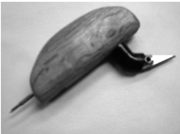
Figura 3 - Taglierina manuale con impugnature in "power grip" Figure 3 - Manual cutting-tool with power grip handle
