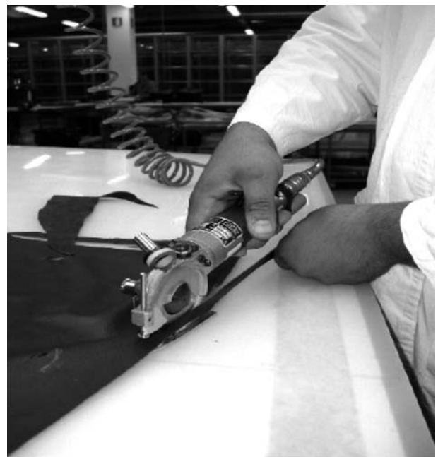
Figura 1 - Taglierina pneumatica a lama rotante Figure 1 - Pneumatic cutting-tool with rotating blade
