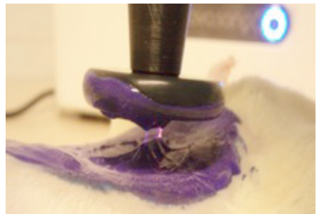
Figure 2 - Set Flat electroporation head, Toluidine blue O solution (moisturizing cream), shaved murine skin, current flow.
