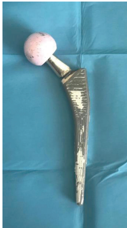
Figure 1b. Case 1. Photograph showing the removed stem, neck and prosthetic head. A complete fracture of the modular neck occurring at the stem-neck junction is visible
