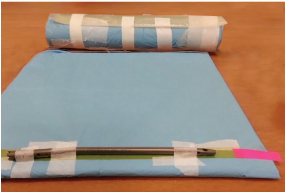
Fig.2 Carbon nail right before being wrapped in water equivalent bolus.
