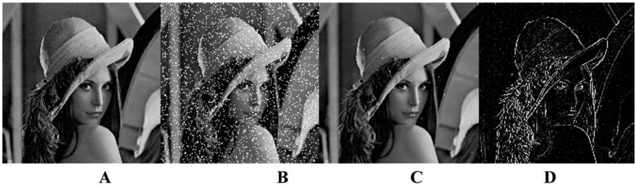
Figure 2. Images of Lena ( left to right ): original (a); noisy (b); preprocessed (c); edges (d).
