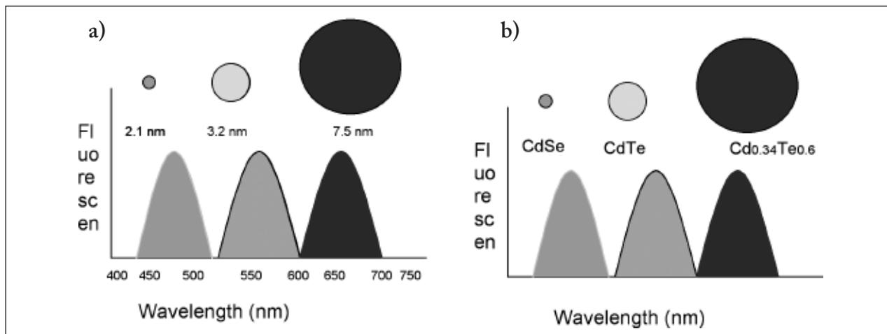
**Figure 2.** Optical properties of binary and alloyed quantum dots. Schematic drawings of three CdSe quantum dots with different diameters (a) and three quantum dots (mean diameter ~5 nm) with different composition (b) and their corresponding fluorescence emission spectra (2)
