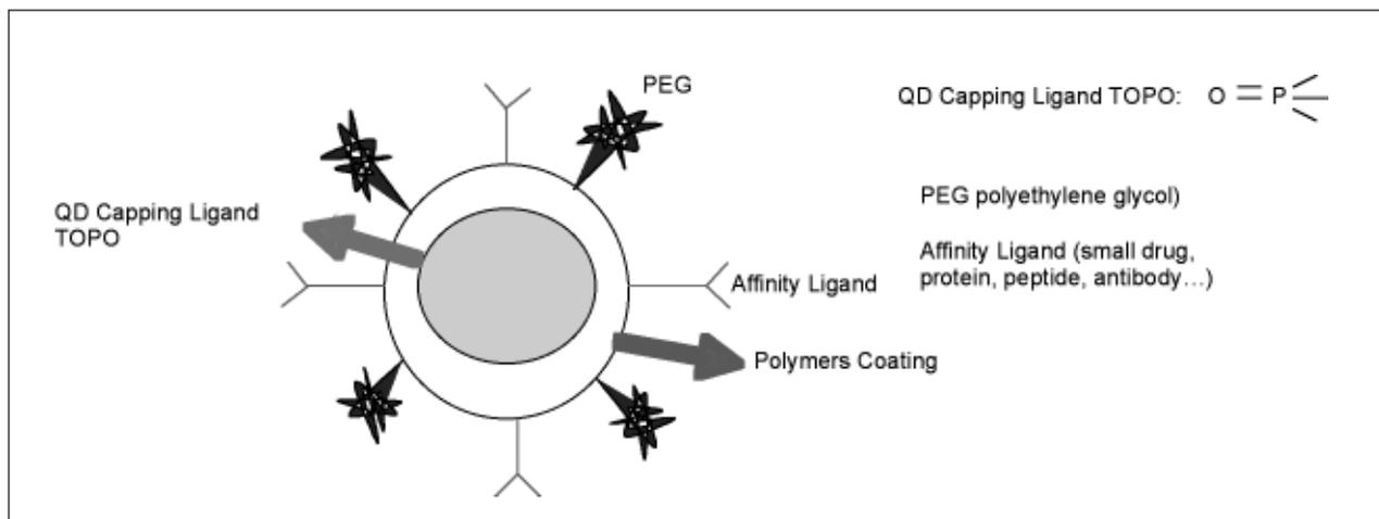
Figure 3. Structure of a Multifunctional Quantum Dot Probe\*
