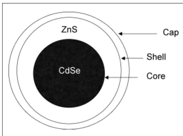
**Figure 1.** Schematic representation of a quantum dot. The cadmium selenide core is surrounded by a shell of zinc sulphide. Finally, a cap can be encapsulate the binary quantum dot by different material such as silica. The diameter of quantum dots ranges between 2-10 nm
