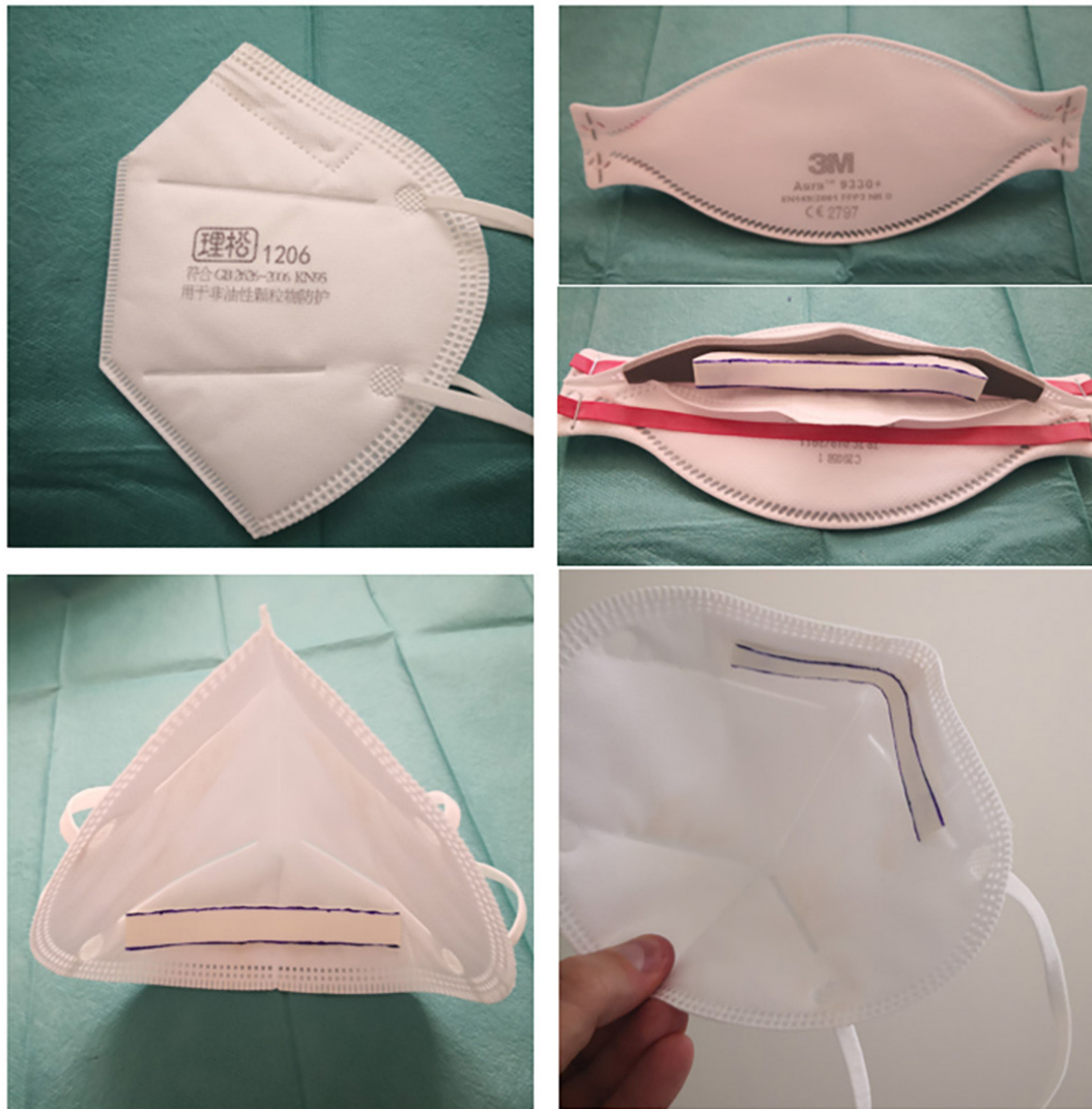
Figure 3. Polyurethane foam modulation for masks
