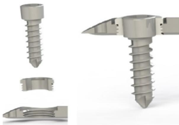
**Figure 1.** Locking coupling mechanism. Three single components of locking mechanism: conically-headed screw, conically shaped bushing inserts with external threads and threaded hole plate (left). Conical screw- bushing insert coupling and threaded bushing insert-plate coupling
