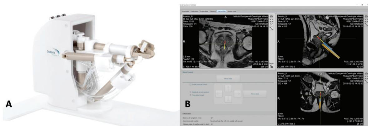
**Fig. 3 “In-bore Robotic System”** – A. Robotic arm; B. The same initial planning images are obtained and sent to the dedicated workstation where the radiologist indicates the needle guide and target lesion locations. On command from the radiologist, the robot then repositioned the needle guide to point in the direction of the lesion.
